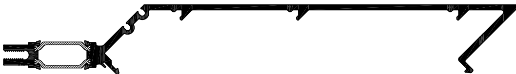
PART# 8200-818 CORNER SPLIT MALE MULLION CAPPED FOR 6-5/8" BACK SECTION
