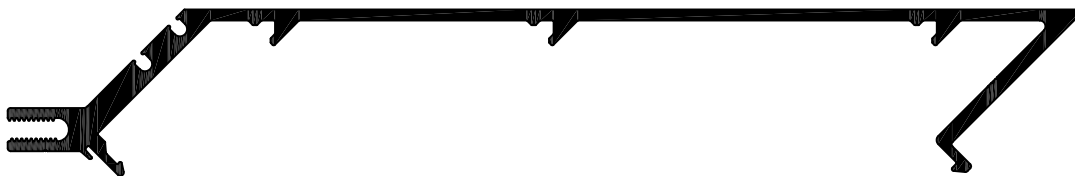
PART#: 8000-018 CORNER SPLIT MALE MULLION CAPPED FOR 6 5/8" BACK SECTION
